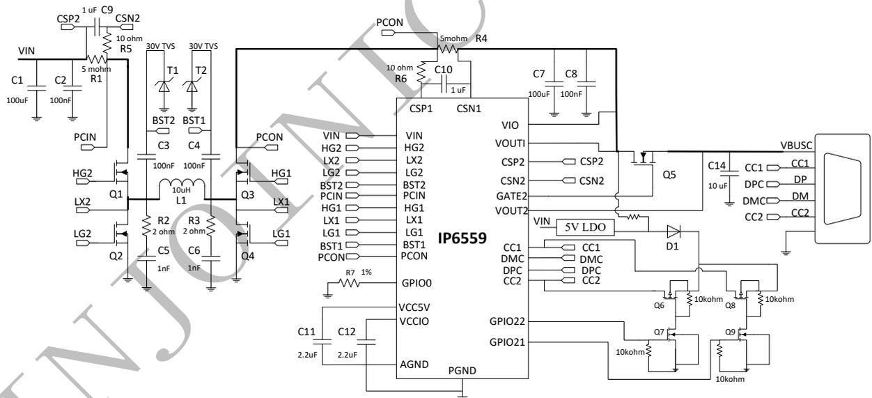
Figure 9. Typical application schematic diagram of IP6559 single C port with EMARK identification output
