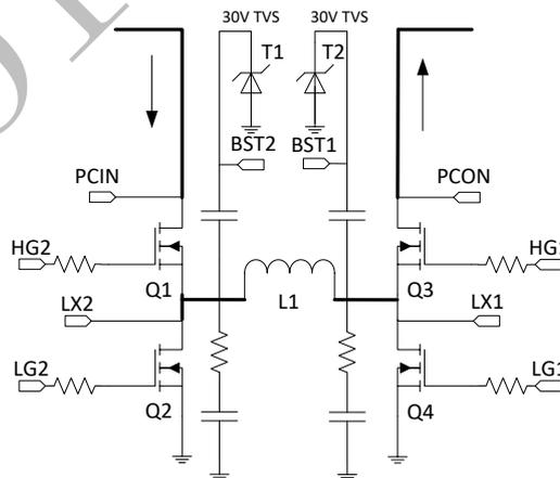
Figure 7. IP6559 MOSFET drive circuit diagram
