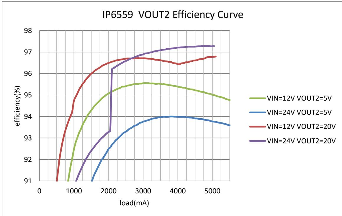
Figure 4. IP6559 VOS1 output efficiency curve
