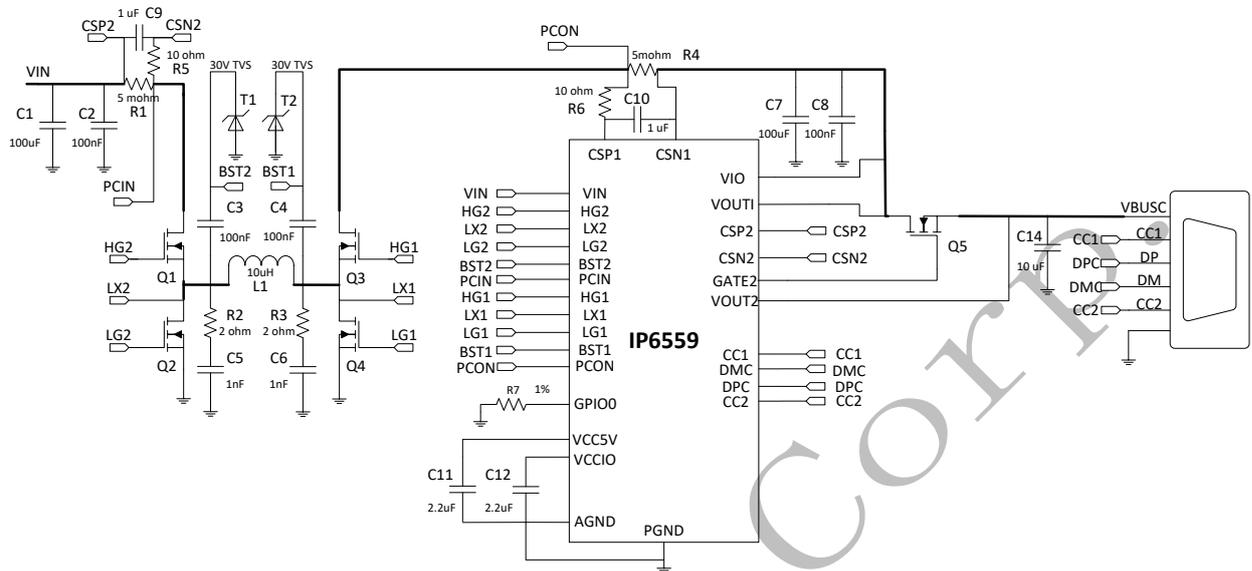
Figure 8. Typical application schematic diagram of IP6559 single C port
