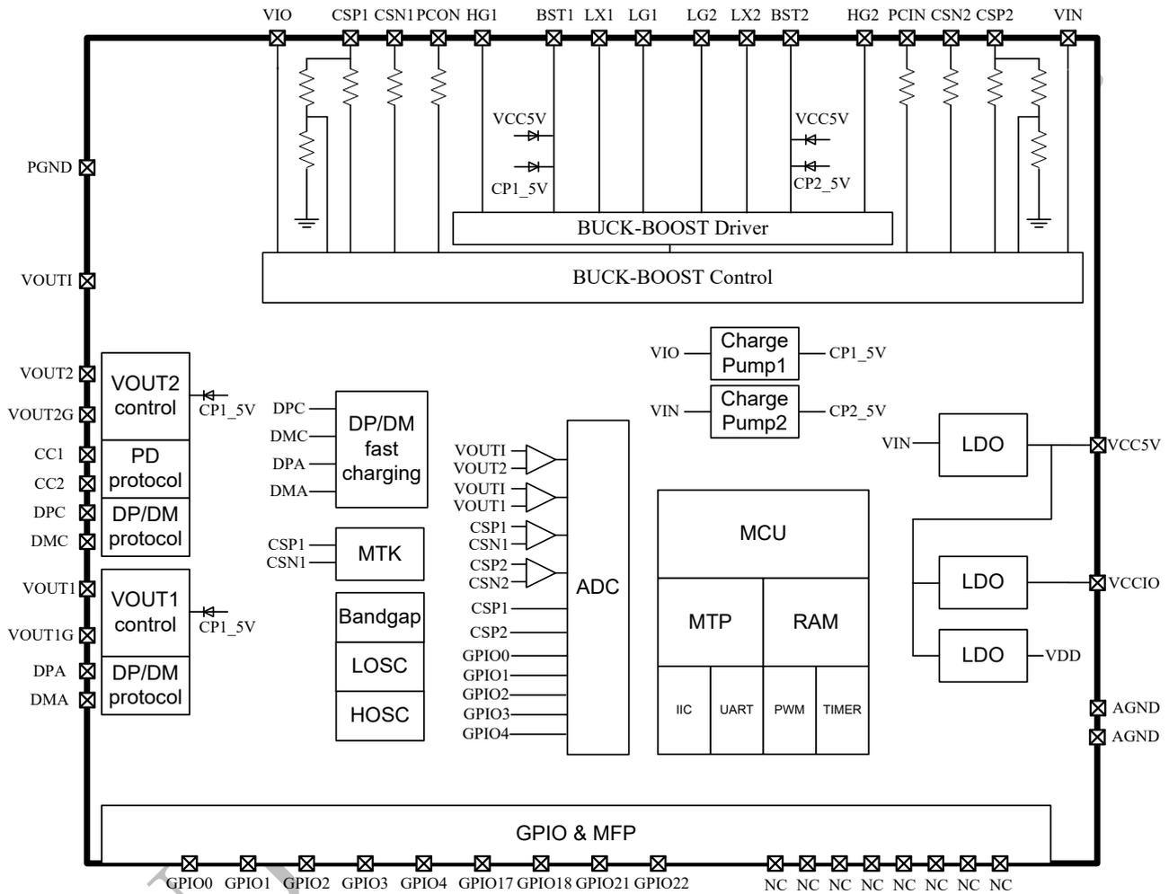
Figure3 IP6559 Internal block diagram
