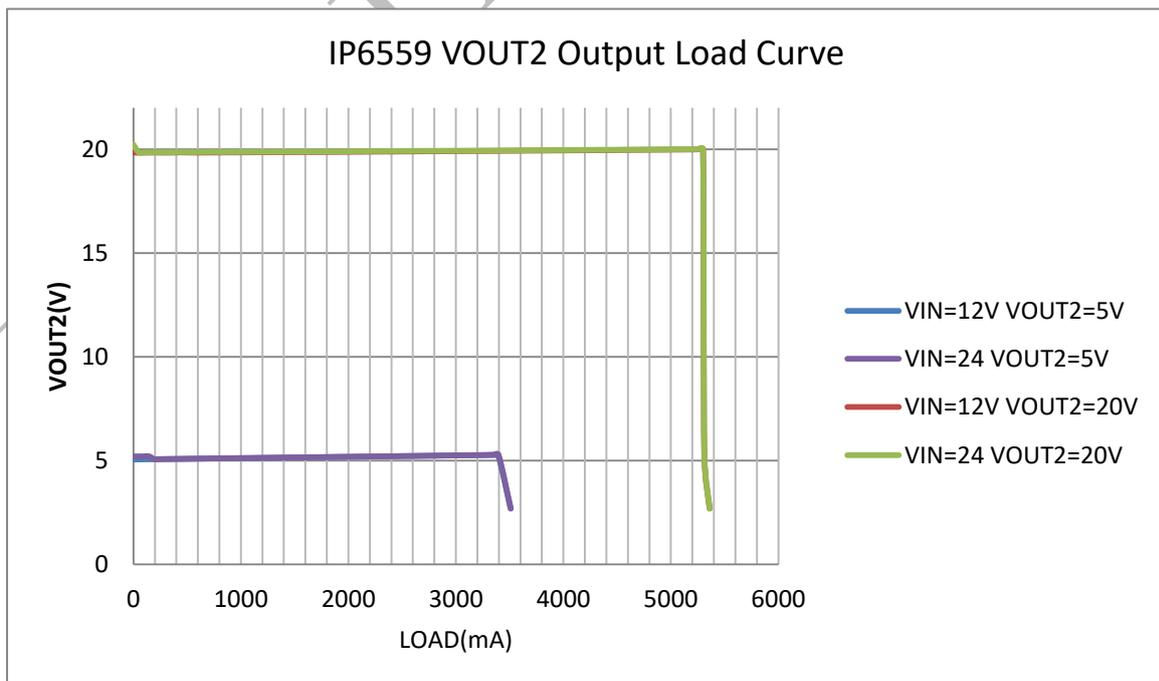
Figure 5. IP6559 VOUT2 output load curve
