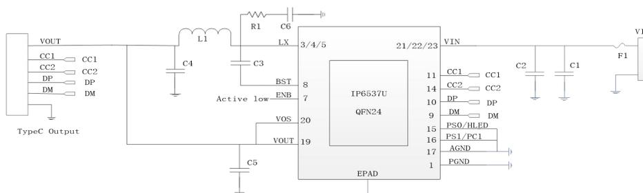
Fig.1 IP6537U Simplified Application Schematic
