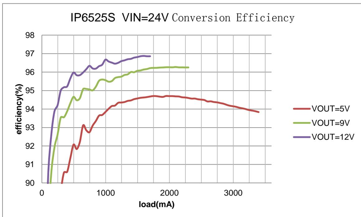
Fig. 4 IP6525S Conversion Efficiency
