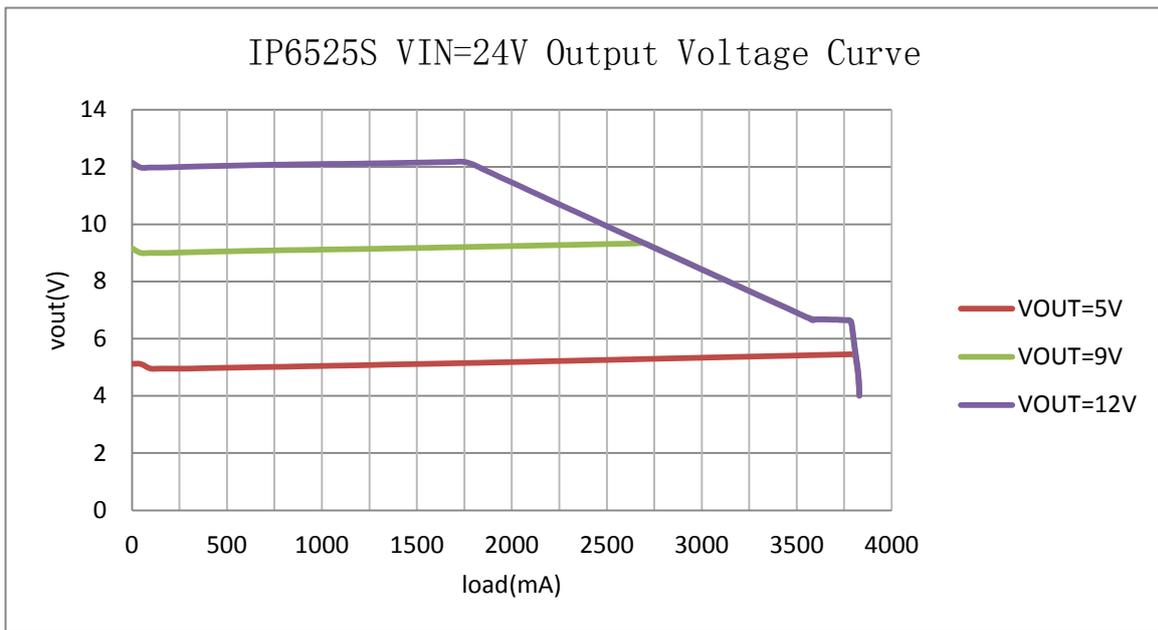
Fig.5 IP6525S Vout-lout curve when VIN=24V
