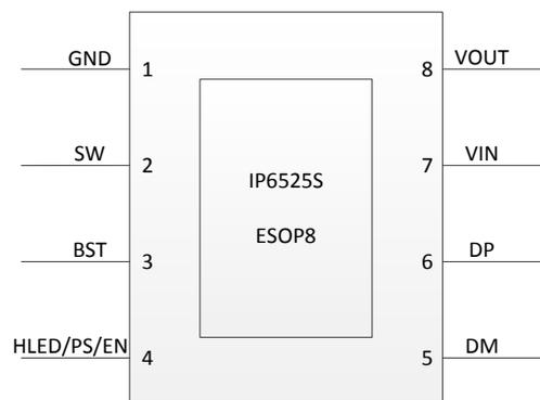
Fig. 2 IP6525S PIN Configuration
