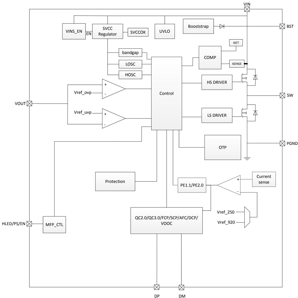
Figure 3 IP6525S Internal block diagram
