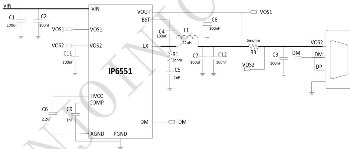
Figure 3. IP6551 Single USB A output ports application schematic diagram
