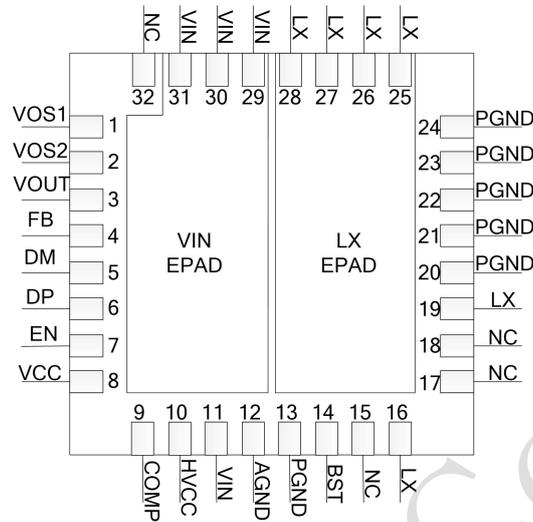
Figure 4.IP6551 (QFN32) Pin functions
