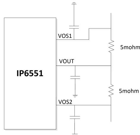
**Figure 8. IP6551 dual output current limiting circuit**
