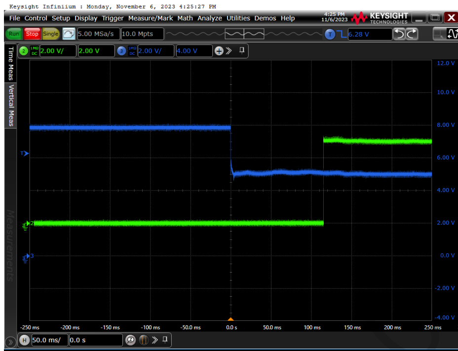
Figure 7 VIN overvoltage recovery (VIN=15V-5V)
