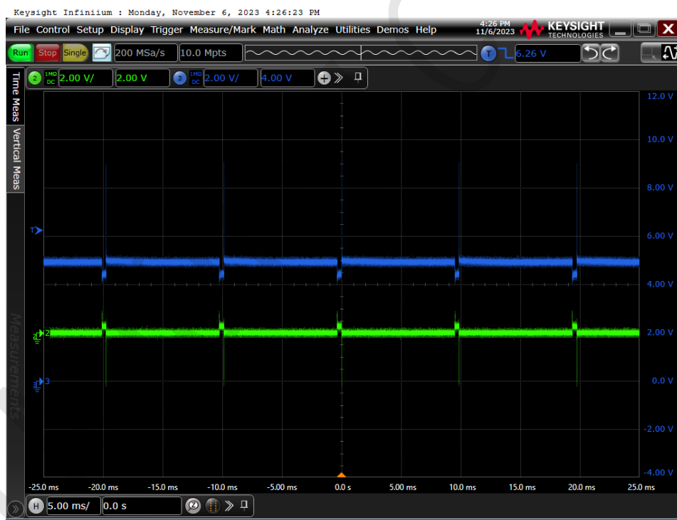
Figure 8 Short circuit hiccup reboot
