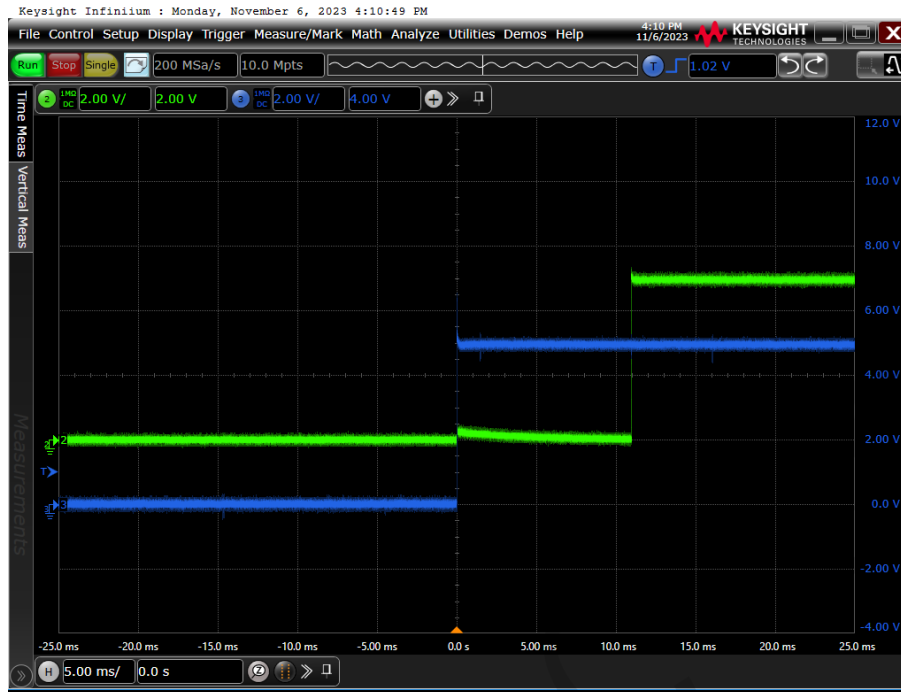
Figure 5 VIN normal power-up start (VIN=5V)
