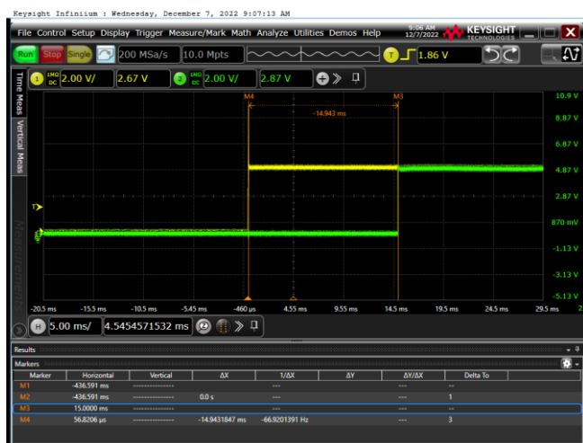
Figure 5 VIN power-on start (VIN=5V)
