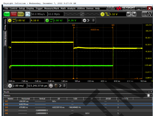
Figure 7 VIN voltage recovery (VIN=7V-5V)
