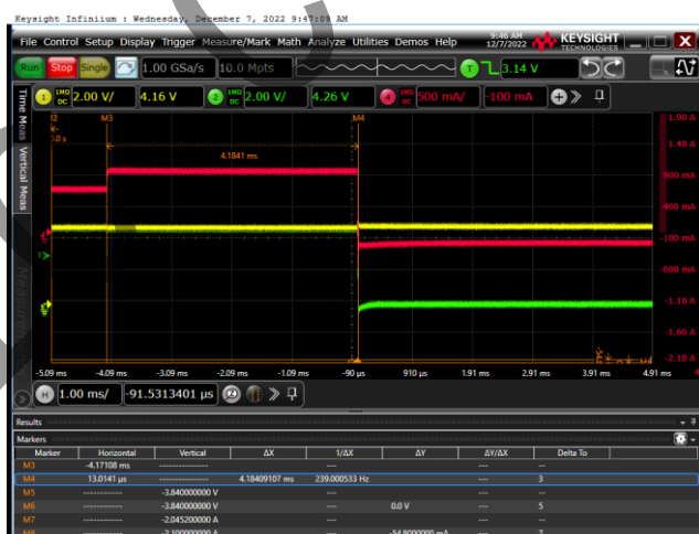
Figure 8 Output overcurrent protection (IOUT=0.9A-1.2A)
