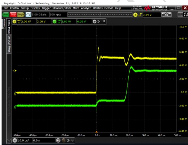
Figure5 VIN power-on start (VIN=5V)
