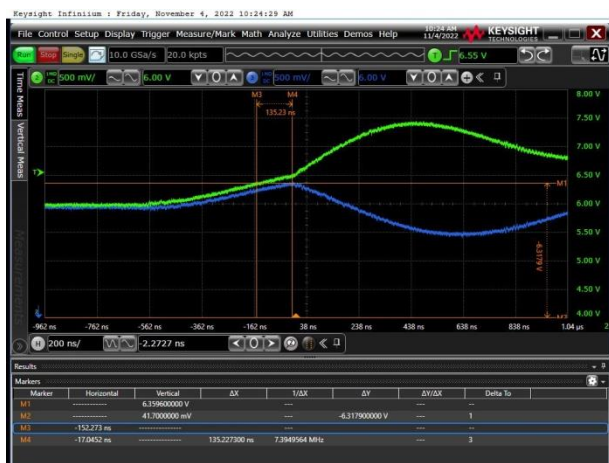
Figure7 VIN voltage protection (VIN=5V-7V)
