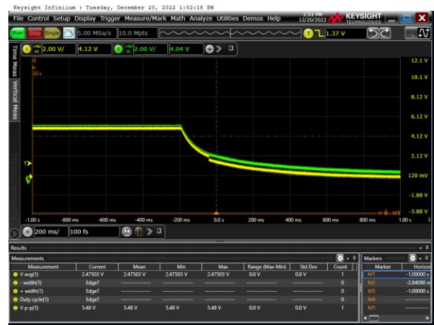
Figure6 VIN powered off (VIN=5V-0V)
