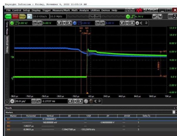
Figure8 VIN voltage recovery (VIN=7V-5V)
